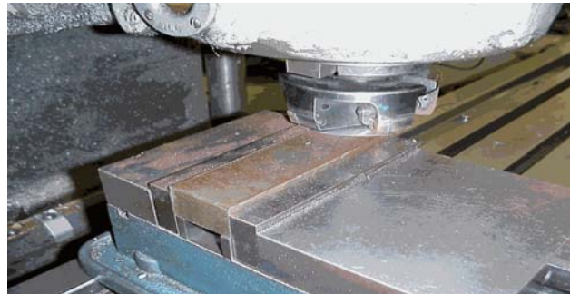
Figure 1. Carbide face mill used on a vertical milling machine.
