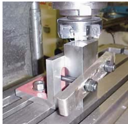
Figure 10: Angle plate being used to machine the end of a long part.
