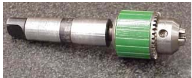
Figure 10 Drill chuck equipped with a Morse taper
