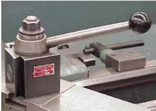
Figure 2 Quick change tool post
